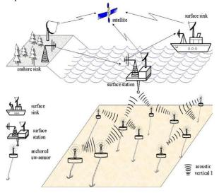
Fig. 5. Architecture for 3D underwater sensor networks.
