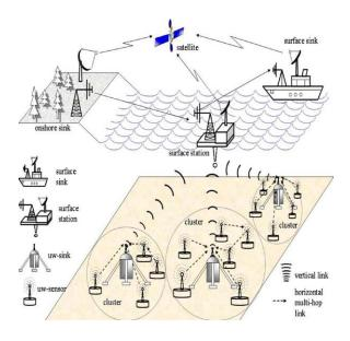
Fig. 4. Architecture for 2D underwater sensor networks.
